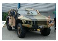
The Army has ordered 1,100 Hawkei Protected Mobility Vehicles – Light (PMV-L) to partially replace the Land Rover Perentie. It is smaller and around half the weight of the Bushmaster. It is able to be carried underslung by the CH-47F Chinook helicopter.
